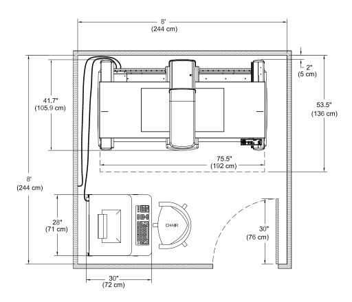
The Horizon DXA system packs a lot of performance into a small footprint. Operating from existing dedicated power sources, the system fits comfortably in an 8' X 8' exam room (8' X 10' for whole body models) and requires no protective shielding or special room preparations.\*
